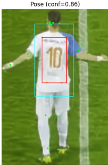
Fig. 2. YOLOv8 pose output (conf=0.86) on a player with jersey number 10. Green dots are detected keypoints. The cyan box is the full player bounding box; the red box is the torso crop derived from shoulder and hip keypoints.
